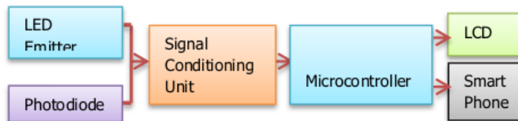
Fig. 3. Diagram block of the blood cholesterol level monitor
